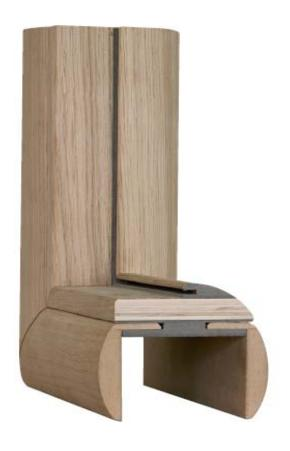
The door frame has very successful combination between elegant design and steady construction. The large tolerance of compensating sills (30 mm) guarantees problem-free assembling even when walls have big deviation. The door frame is produced in six basic dimensions, which makes it appropriate for wall thickness from 85 mm to 215 mm. Door frame is produced in various designs of PP foil and also high gloss white, veneer oak and veneer oak fine line.
