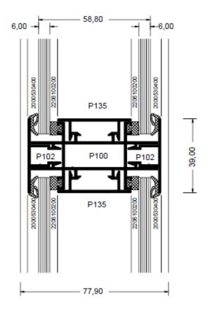
Flush glazing with axial junction joint
